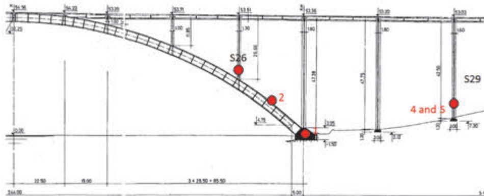
Fig. 1: Positions of the corrosion sensors on the small arch of the Krk bridge
