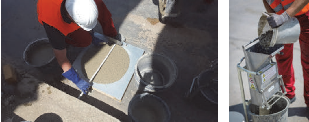
Fig. 5: Determination of the flow spread (left) and separation of steel fibers from the fresh concrete (right)
