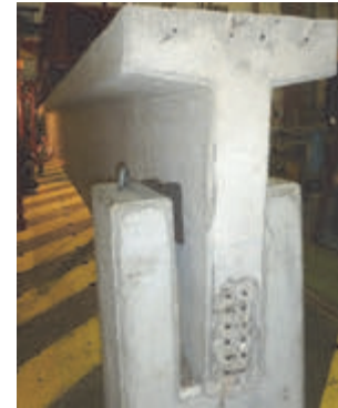
Fig. 2: Shear loading arrangement of beam T90 and picture of the T90 beam on the test stand
