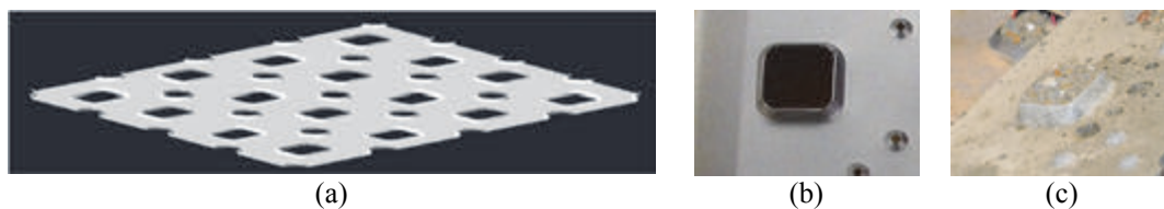
Fig. 1: Reinforcing system of a perforated steel sheet (a) in 3D view, (b) detail of a bulged perforation, & (c) concrete corbel formed within the bulged openings of the steel sheet (Apostolidi & Strauss, 2014)
