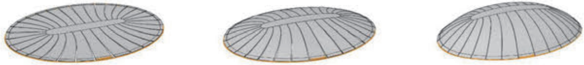
Fig. 1: Construction of a concrete shell originating from a thin flat hardened concrete plate by the aid of an air cushion placed underneath the plate and tensioning a post-tensioning tendon mounted at the circumference
