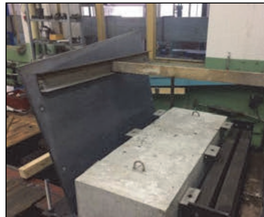
Fig. 7: Test of load bearing capacity of the left thin wall – a way out direction
