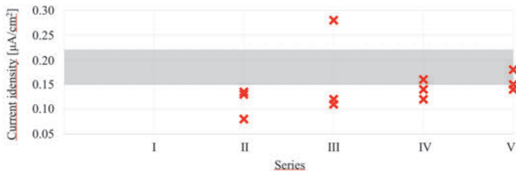
Fig. 4: The values of corrosion current density obtained from results of all types of the analyzed concrete
