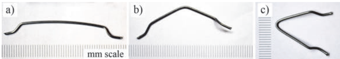
Fig. 2: Steel fibres prepared to pull out test, a) initial shape, b) deformed shape, c) “U” shape
