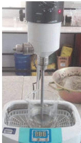
Fig. 1: Mixture of cement, CNTs and isopropanol in the ultrasonic bath being mechanically agitated
