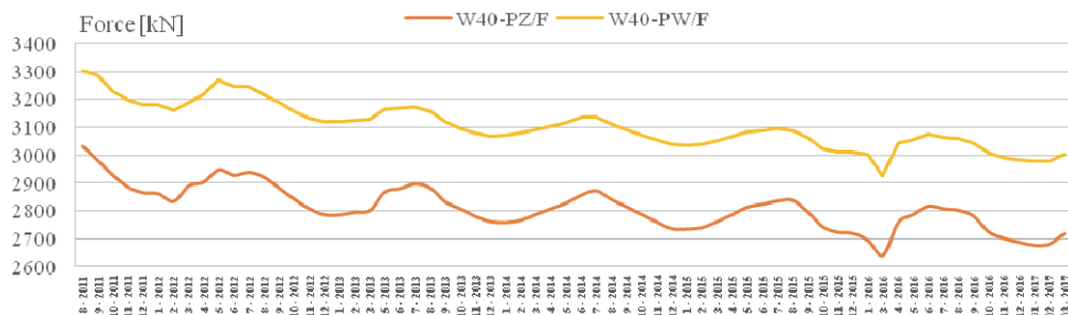
Fig. 5: The monthly average forces in case of the longest stay-cables W40-PZ/F and W40-PW/F
