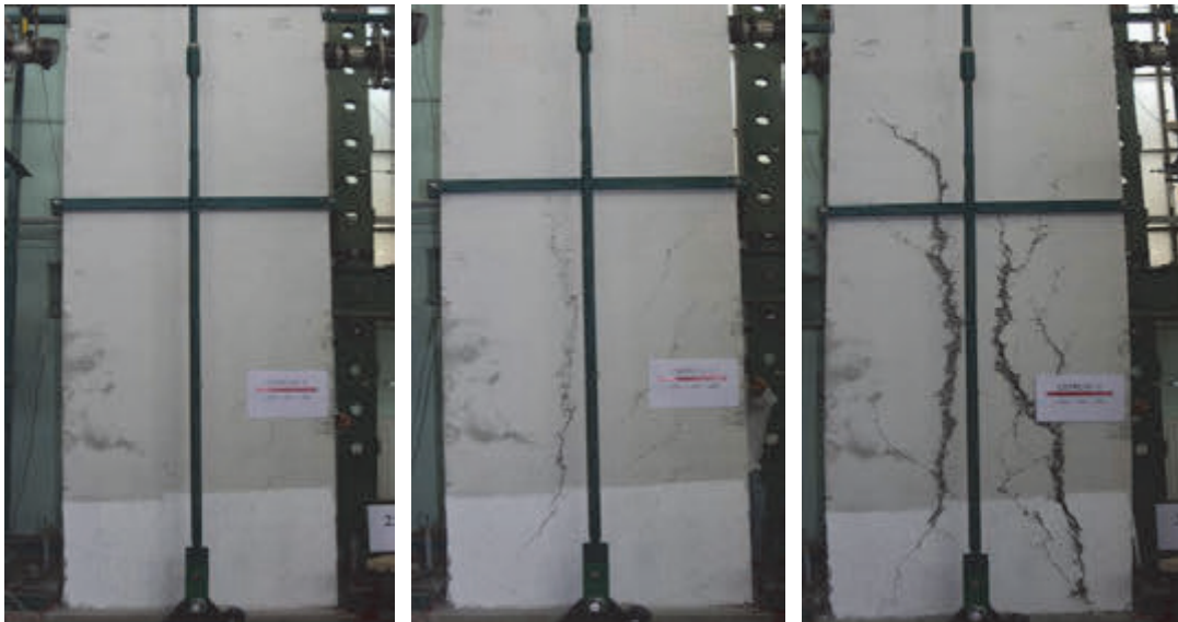
Fig. 5: Type of failure modes of steel-concrete composite walls
