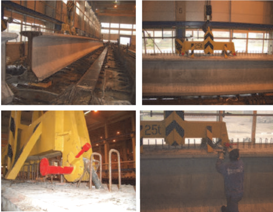
Fig. 4: Bridge girder production, transportation within the plant
