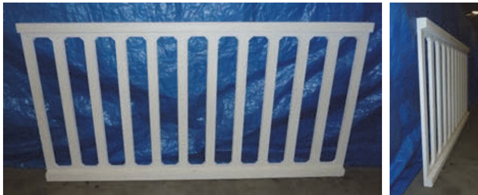
Fig. 2: UHPC panel with longitudinal reinforcement
