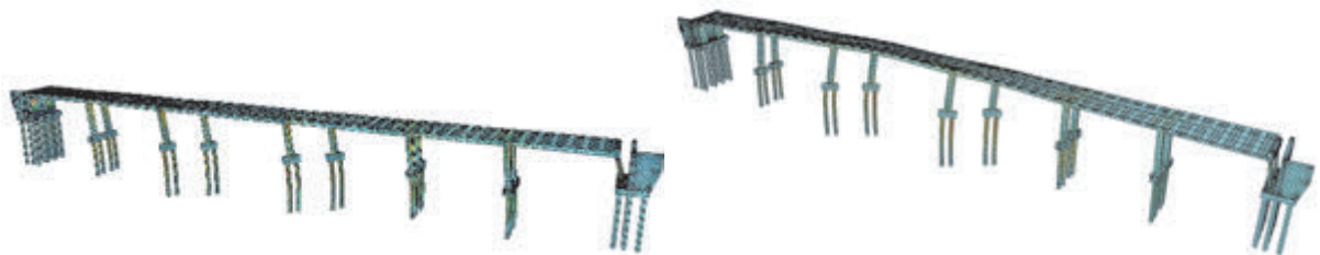
Fig. 9: The FE-Model – seismic evaluation
