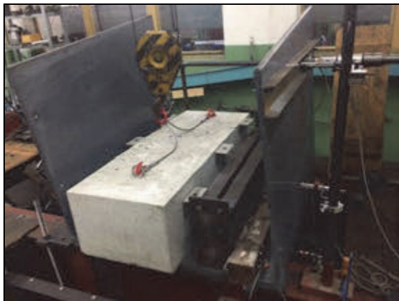
Fig. 6: Test of load bearing capacity of the right thin wall – an inward direction
