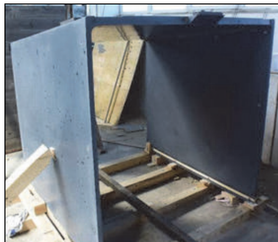
Fig. 3: Preliminary mock-up after the demolding
