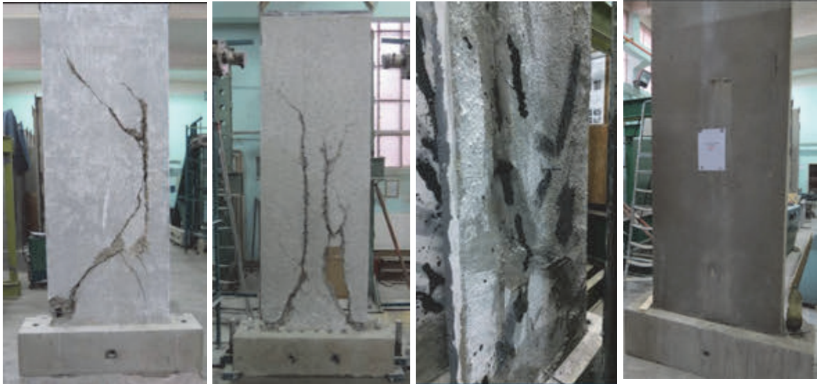
Fig. 6: Level of degradation stage, retrofitting and strengthening walls with FRCC
