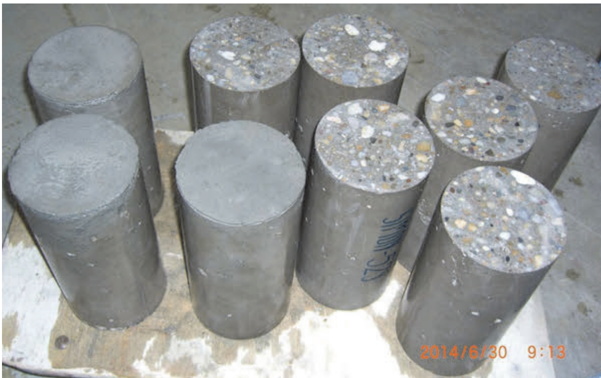
Fig. 6: Sample cylinders, which have the size of Ø150×300 mm, until the age of 28 days kept under water, cupped with cement mortar or polished on their compressed surface
